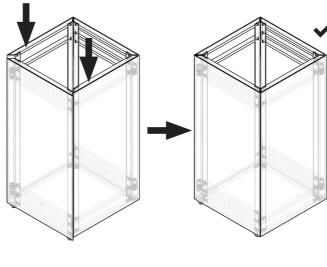
Step 6: Push two side panels down applying even pressure to each side.
