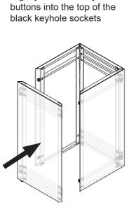
Step 5: Mate back panel to the two side panels ensuring yellow buttons are inerted up into black keyholes.
