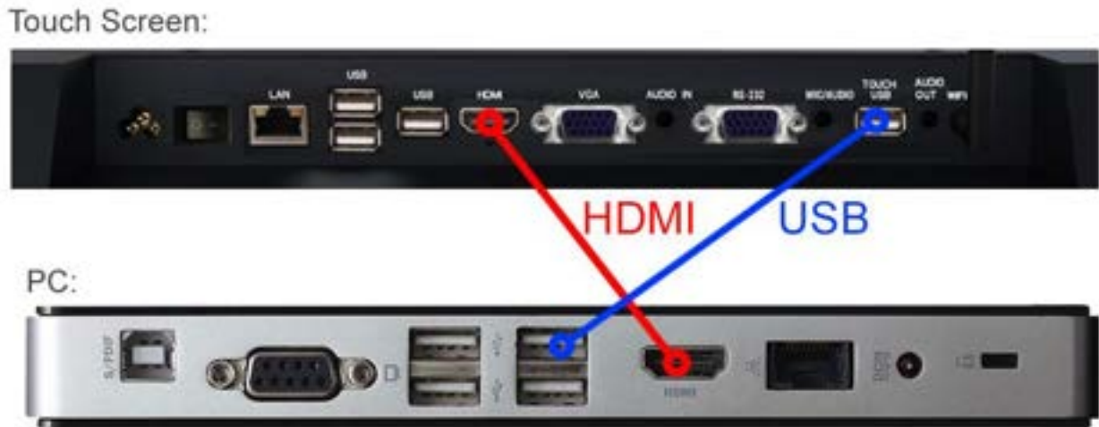
Figure 1 Screen to PC Connections
