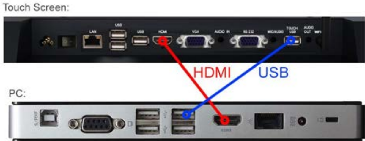
Figure 4 Screen to PC Connections
